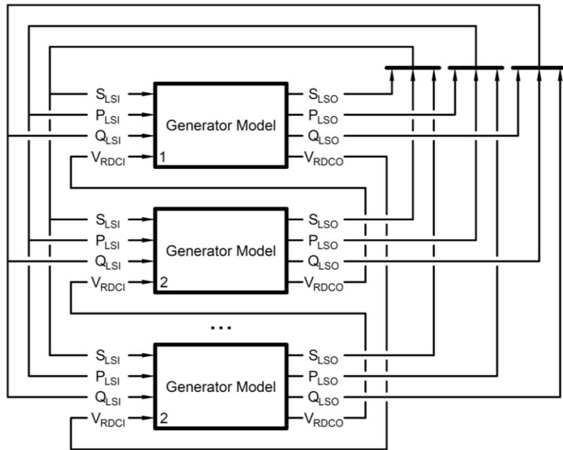
**Figure 1: Load sharing input and output signals for an arbitrary number of generator models.**
