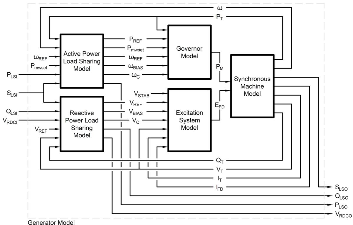
**Figure 2: Active and reactive power load sharing models and their inputs and outputs in the generator model. Note: changes of base are not shown in this figure.**
