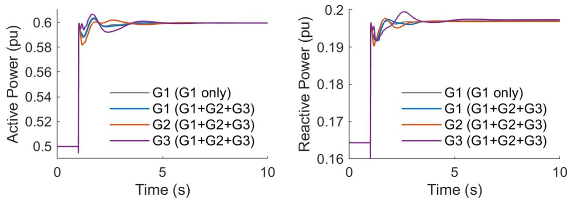
**Figure 7: Active and reactive power response G1, G2, and G3 for a step load as compared to G1 only.**
