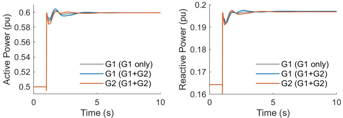
**Figure 6: Active and reactive power response of G1 and G2 for a step load as compared to G1 only.**
