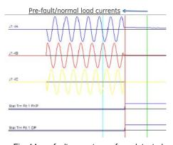
Fig. 14 pre-fault current waveform detected
