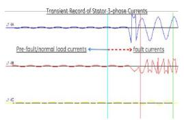
Fig. 12 Damaged motor transient record of stator currents.
