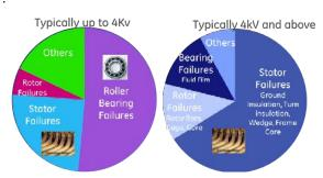
Fig. 1 Electric machine failures-typical [1],[2].
