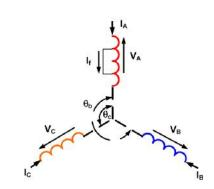
Fig. 5 Stator inter-turn fault illustration in 3- phase winding of the machine
