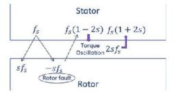
Fig. 8 Theoretical representation of induced rotor fault signature in stator currents
