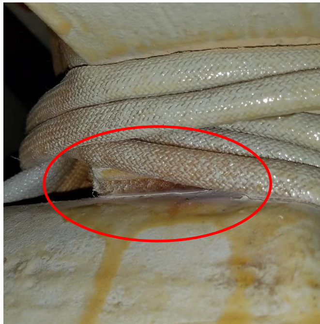
Figure 10 – Dusting Between the Rope Lash and Circuit Ring near 1:00 Top Jumper in 2019
