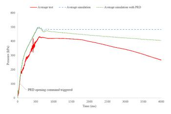
Figure 8: Tank pressure comparison with PRD
