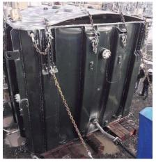
Figure 9: Rupture at the tank cover
