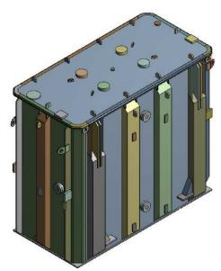
Figure 1: Geometric model of the transformer tank under consideration
