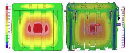
**Figure 6:** Permanent displacements after the design energy level test (left: simulation; right: scan measurement)
