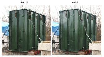
Figure 4: Tank deformation before and after the design energy test
