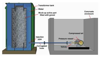
Figure 3: Schematic of gas injection system with respect to the tank
