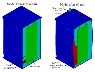
Figure 7: Tank cross section model for explicit dynamic simulation
