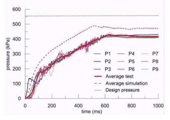
Figure 5: Design energy level test pressure measurements
