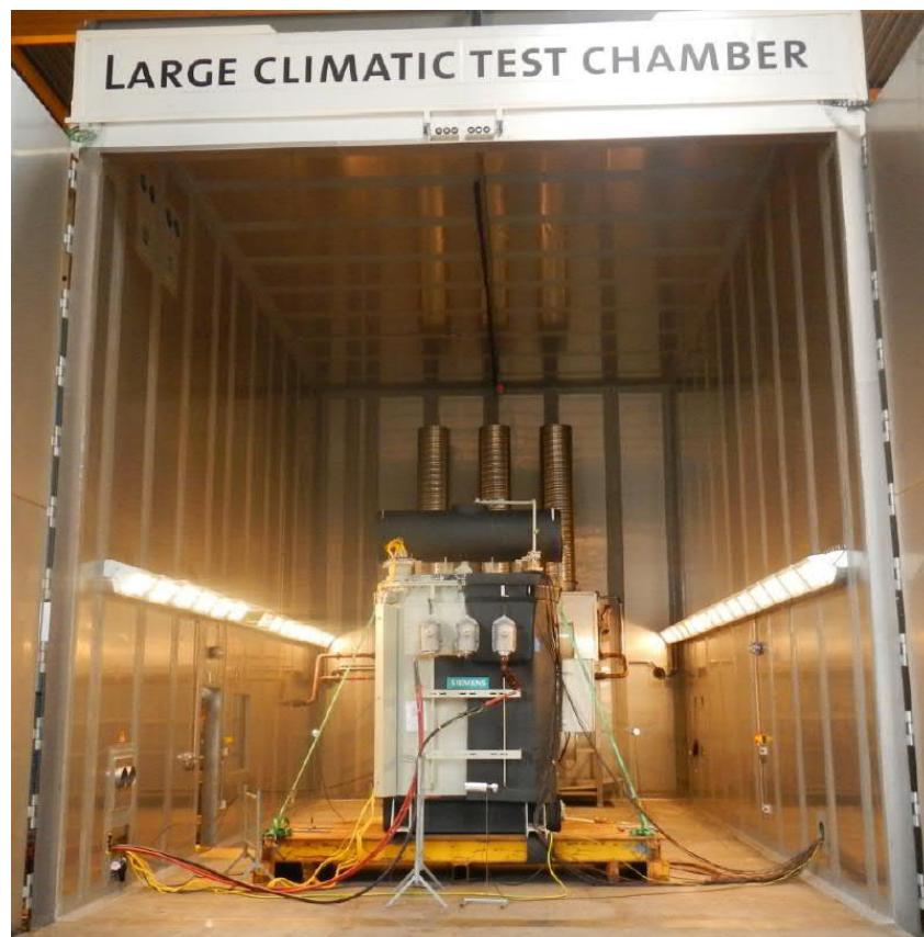
Picture 1: Test object inside test chamber with walls partially insulated
