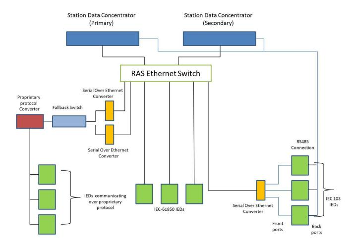
Figure 1 Connection diagram of different Protocol Relays at Substation
