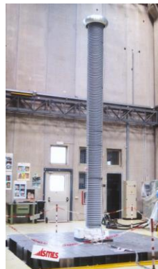
Figure 8: RC 500 VG during seismic test
