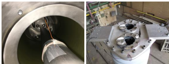
Figure 3: a) Ignition arrangement for internal arc test according to IEC 61869-1; b) properly triggered rupture disks for 245 kV Clean Air voltage transformers
