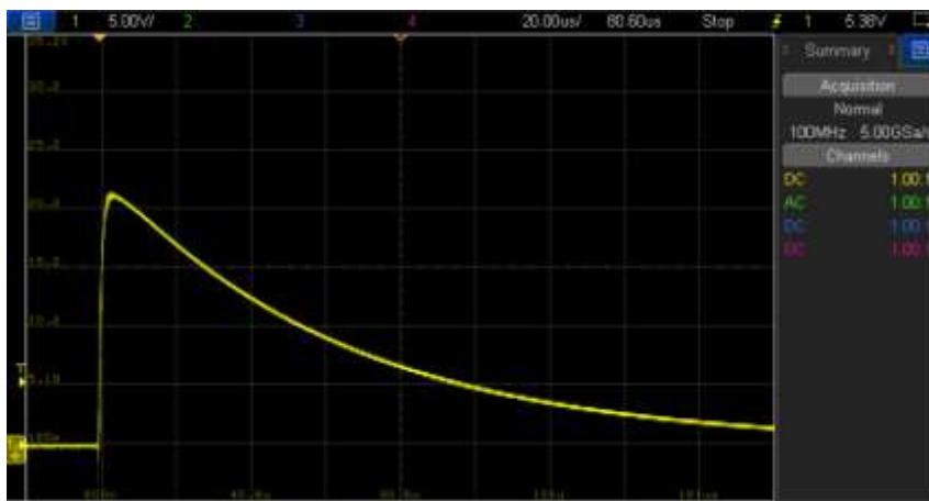
Figure 9 Low voltage output of FTT with 210V peak amplitude. X axis is 20 µseconds per division and Y axis is 5 volts per division
