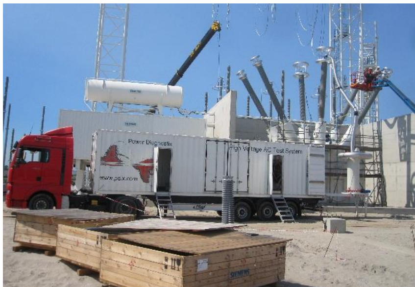
Figure 6: Inverter based three-phase mobile test system for on-site testing.
