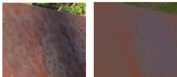
Fig. 6. Original corroded image (left) and the image’s reflectance derived from global sparsity (right)
