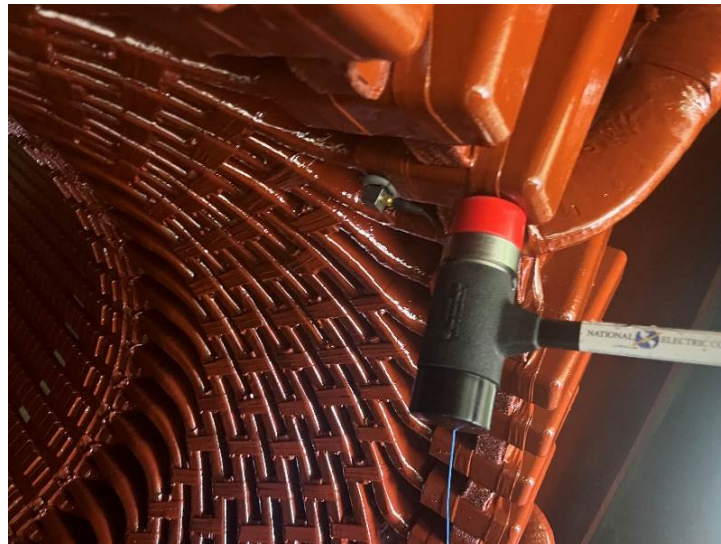
Figure 1: Exciter End – Impact Test Example at Series Connection – Photo courtesy of NEC
