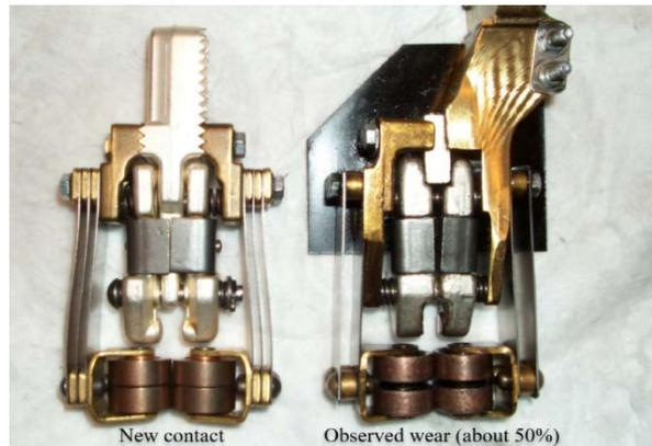
**Figure 1:** New contact and contact with observed wear of about 50%.
