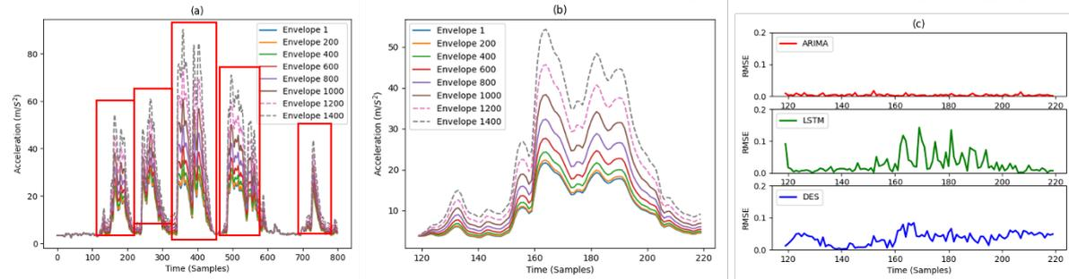
**Figure 4:** (a), (b) The training and predicted envelopes (dashed lines) by combined model applied on D2 dataset and (c) RMSE data used to select the best forecasting model for each sample of graph (b)
