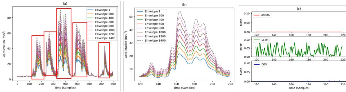
**Figure 3:** (a), (b) The training and predicted envelopes (dashed lines) by combined model applied on D1 dataset and (c) RMSE data used to select the best forecasting model for each sample of graph (b)
