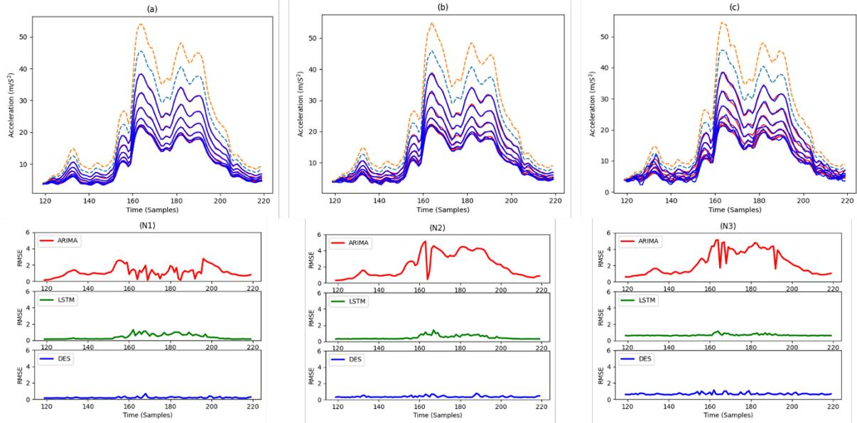
**Figure 6:** The training and predicted envelopes (dashed lines) by combined model applied on D2 dataset with (a) N1, (b) N2, and (c) N3 noise level. Simulated envelopes without noise are in red and simulated envelopes with noise are in blue. RMSE data used to select the best forecasting model for each sample are shown below the graphs.
