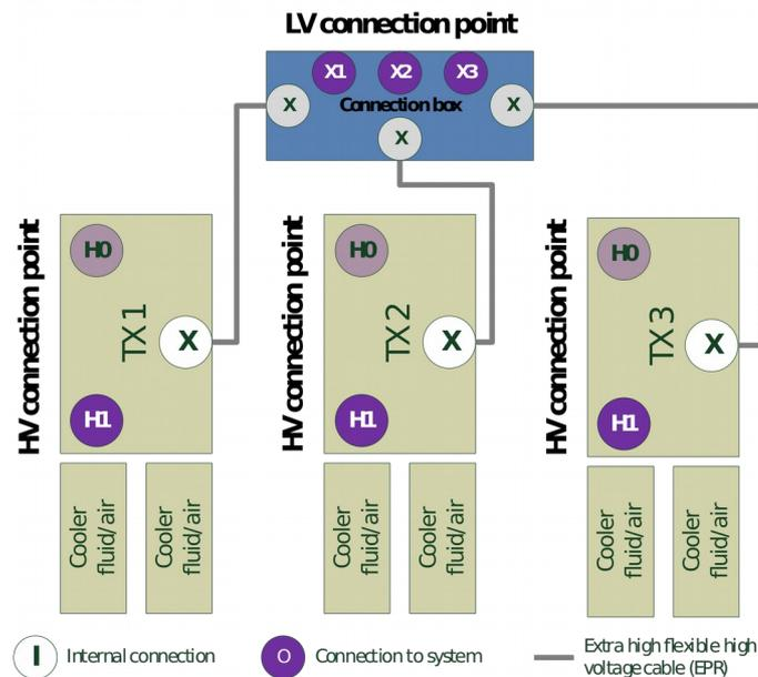
Figure 2 - Connection diagram
