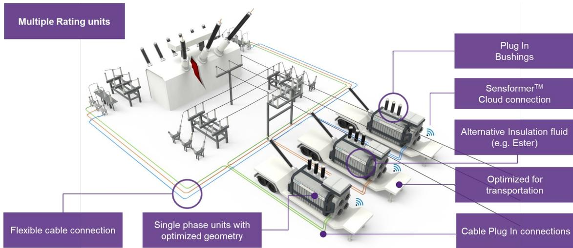
Figure 1 - Schematic arrangement of Siemens Energy's resilience concept [2]
