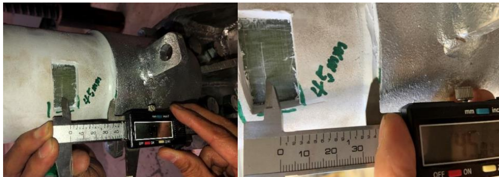
Figure 11. End fitting slippage measurement before and after cyclic load tests.
