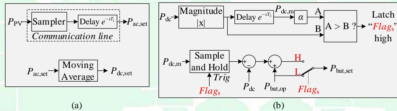
Power set point calculators with local active power measurements (a) rectifier (b) inverter.
