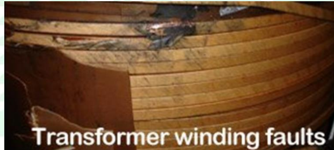
Bad insulation paper due to partial discharge
