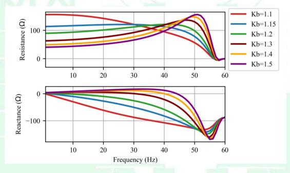
TCSC behaves more like a capacitor at sub-synchronous frequencies at low boost factors,
