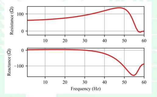
TCSC presents a resistance at sub-synchronous frequencies and acts as an inductor in the frequency range from 1-30Hz
