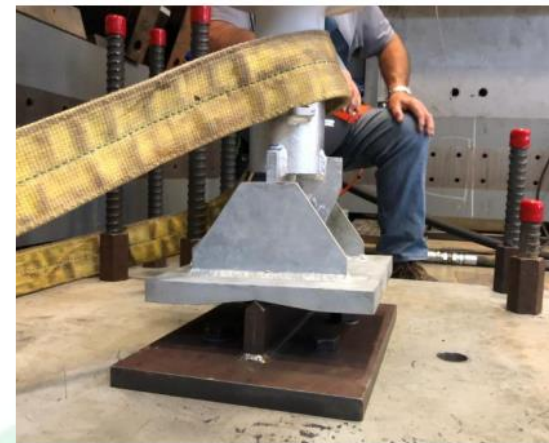
Post insulator ultimate compression capacity test
