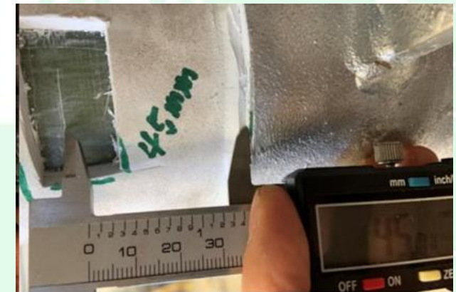
Slippage measurements before and after Cyclic Test
