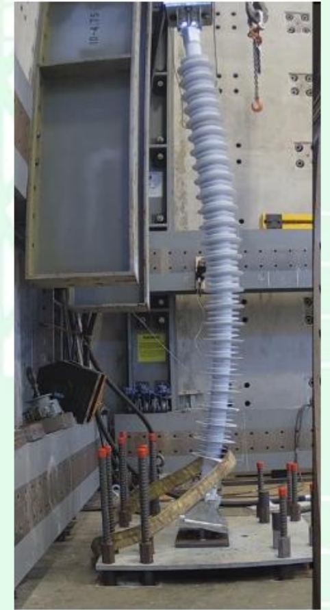
Post insulator ultimate compression capacity test
